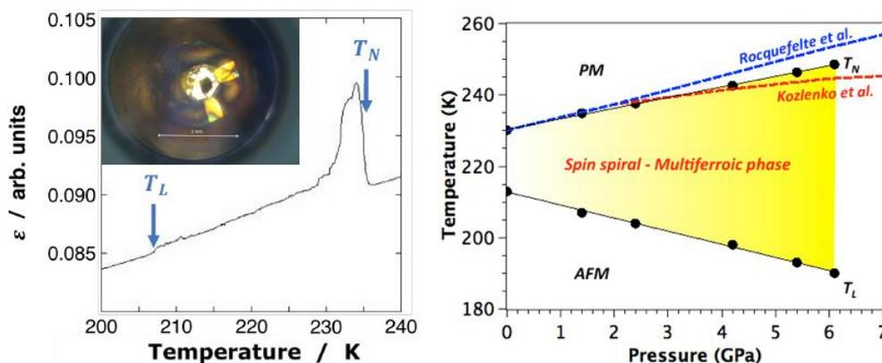
**Figure.** Left: Dielectric constant (capacitance) measurement on a single crystal of CuO under a pressure of 1.4 GPa. At  $T_N$  a large jump of the signal occurs. At  $T_L$  a much smaller but still clearly visible anomaly is seen. The inset shows the sample of CuO pressurized in the diamond anvil cell for dielectric constant measurements seen through the diamonds. Right: Schematic representation of our recent measurements of  $T_N$  and  $T_L$  (black dots) under high-pressure.
